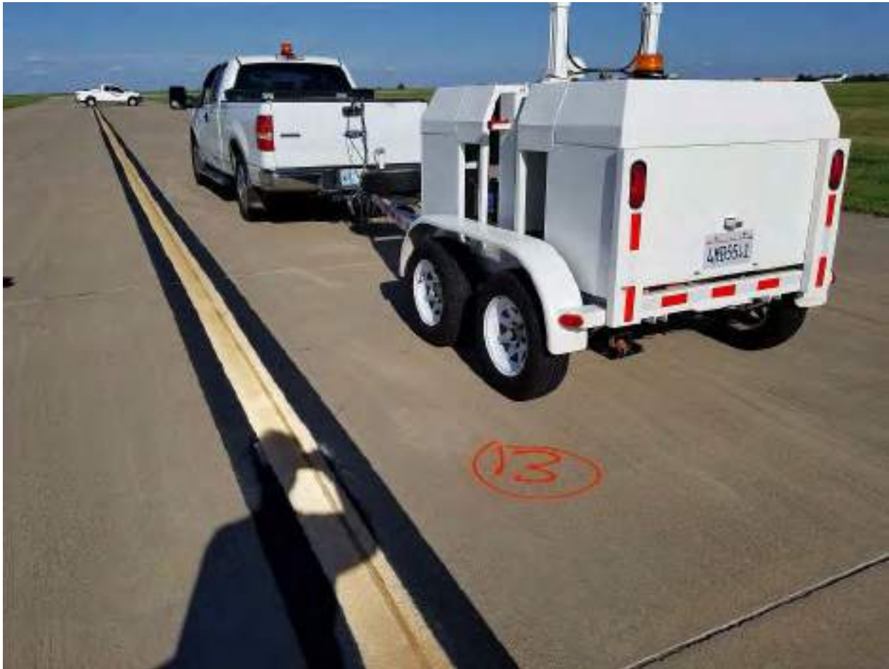
Photo 3 – Typical FWD Tests at Center Lane of PCC Slab
