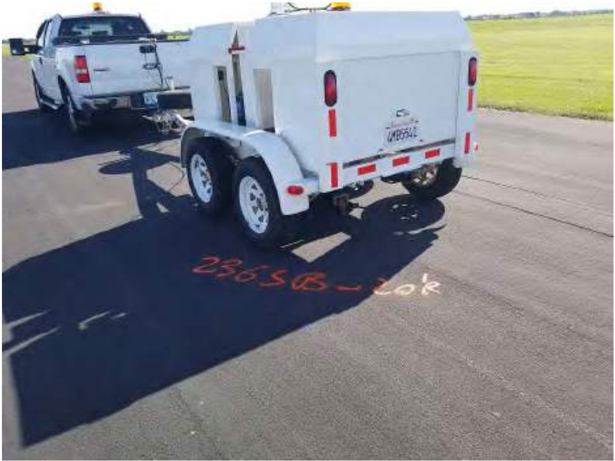
Photo 2 – Typical FWD Tests at Asphalt Pavement with 20 feet Offset Right from Centerline
